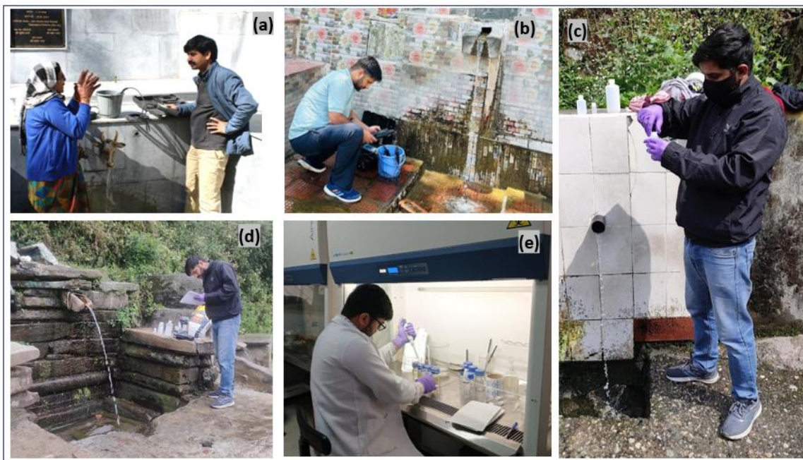
Fig. 4.2 Field and laboratory activities for spring water assessment: (a) community interaction during site visit, (b) on-site measurement and sampling, (c) sterile water sample collection, (d) field testing at a natural spring, and (e) laboratory analysis of samples.
